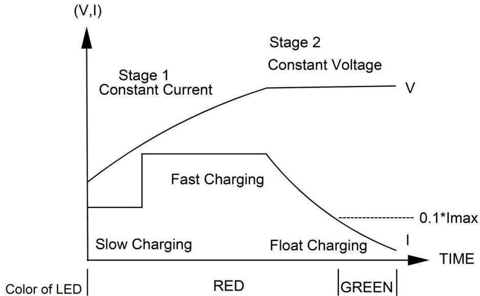
\*Note: This charging curve is for Li-Ion battery.
